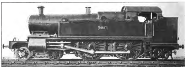
Fig. 5059. Ten-Wheel, Four-Coupled Tank Locomotive. Great Western Railway. Cylinders 18 in. x 30 in.; Working Steam Pressure 195 lbs. per sq. in.; Total Heating Surface 1,517.89 sq. ft.; Weight on Drivers, 64,960 lbs.; Total Weight 168,000 lbs.
